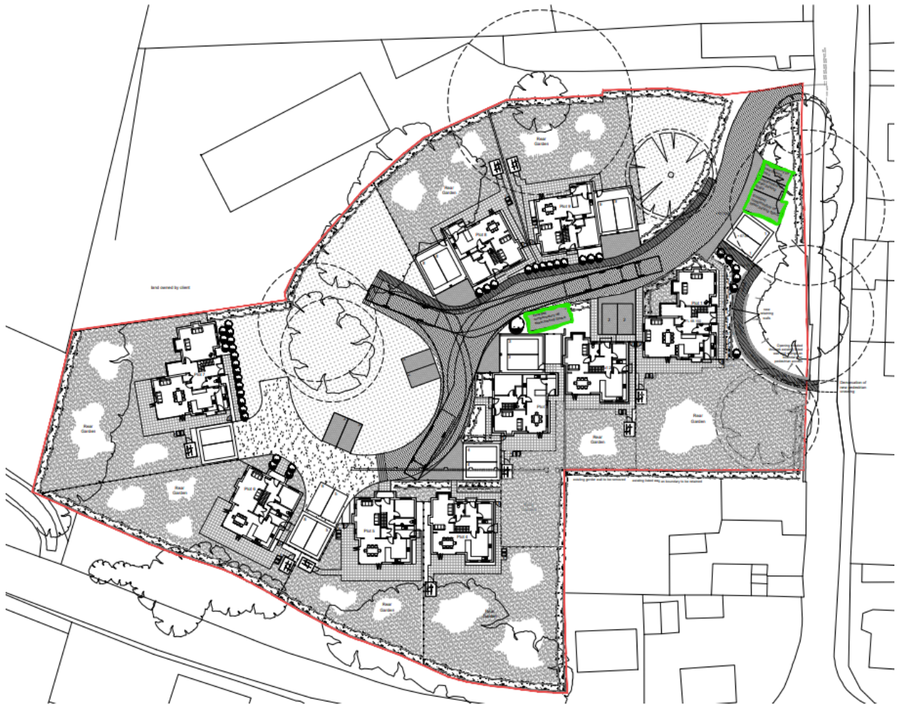
Figure 1 - Amended Proposed Site Layout (4 no. compensatory parking spaces highlighted in green)
